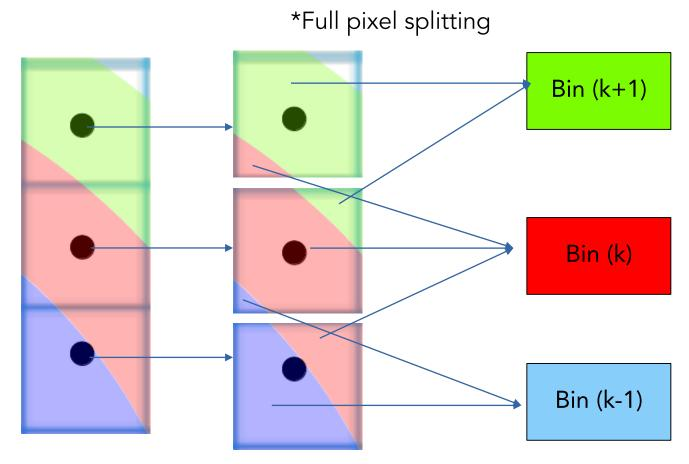
Each bin is the sum of the intensities of different pixels multiplied by a weight component between 0.0 and 1.0.
